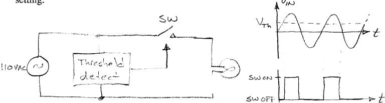
The first method is simpler, but a significant amount of power is wasted in the variable resistor. The second method is close to what is used in solid-state dimmer switches; they typically use solid-state switches known as Triacs (see Chapter Two) which are turned on for some portion of each cycle of the sine wave.
