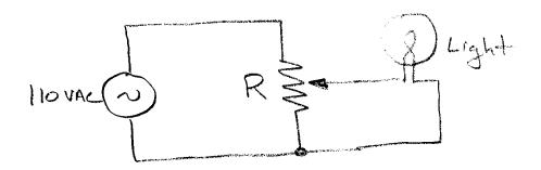
A second method would be to use a variable threshold and only allow current to flow in the light when the input voltage is above the threshold. For this method to work we need a circuit to generate the threshold, which must depend on the setting of some control, and we need an electronically controllable switch. A simplified diagram is shown below along with the input waveform and an example of when the switch would be on for a given threshold setting.
