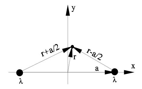
(a) By symmetry, the electric field of a long straight wire is perpendicular to the wire. Its magnitude a distance r from the wire is given by
