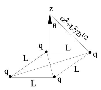
(a) The four point charges q are located at the corners of a square with sides of length L. The distance from each charge to a point z above the square, on the perpendicular axis of the square, is  $\sqrt{z^2 + L^2/2}$ . The horizontal fields cancel, and the magnitude of the vertical field is given by
