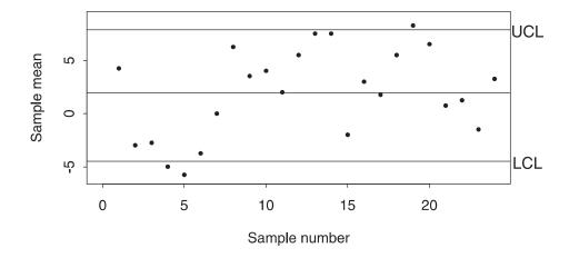
Figure 1.2: X-bar chart for crank bore diameter. Exercise 1.8
