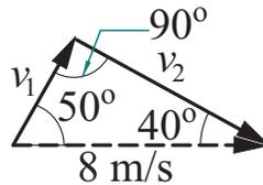
$$v_1 = 8 \sin 40^\circ = 5.14 \text{ m/s} \blacktriangleleft \quad v_2 = 8 \sin 50^\circ = 6.13 \text{ m/s} \blacktriangleleft$$
