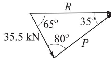
$$\frac{P}{\sin 65^\circ} = \frac{35.5}{\sin 35^\circ} \quad P = 35.5 \frac{\sin 65^\circ}{\sin 35^\circ} = 56.1 \text{ kN} \quad \blacktriangleleft$$
