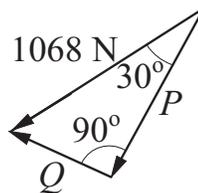
$$\text{Component parallel to } AB : P = 1068 \cos 30^\circ = 924.9 \text{ N} \blacktriangleleft$$
