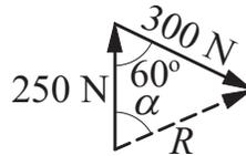
First compute the resultant  $\mathbf{R}$  of the two known forces. The smallest required  $\mathbf{F}$  has the same direction as  $\mathbf{R}$  and its magnitude is  $500 \text{ N} - R$ .
