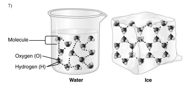
The type of bond indicated by the dotted lines in the accompanying figure is a hydrogen bond.
